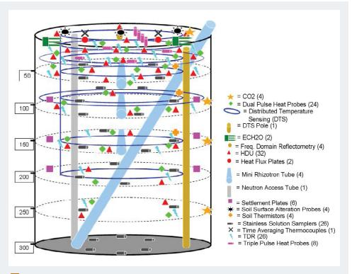
Sensors to measure moisture content, temperature, heat, and CO2 inside of the SEPHAS lysimeter soil.
