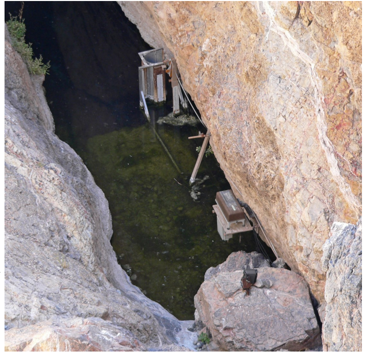
Devils Hole as seen from above. The equipment shown is used to measure the water level.
