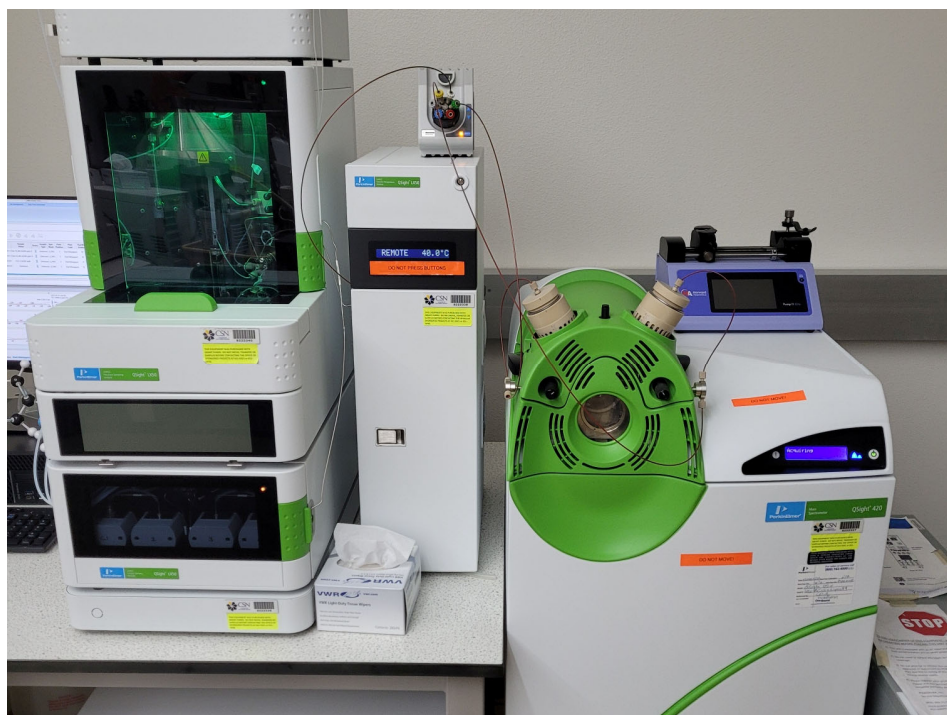
The LC-MS/MS at the CSN West Charleston Campus used to analyze the water samples for ECs (photo courtesy of Douglas Sims).
