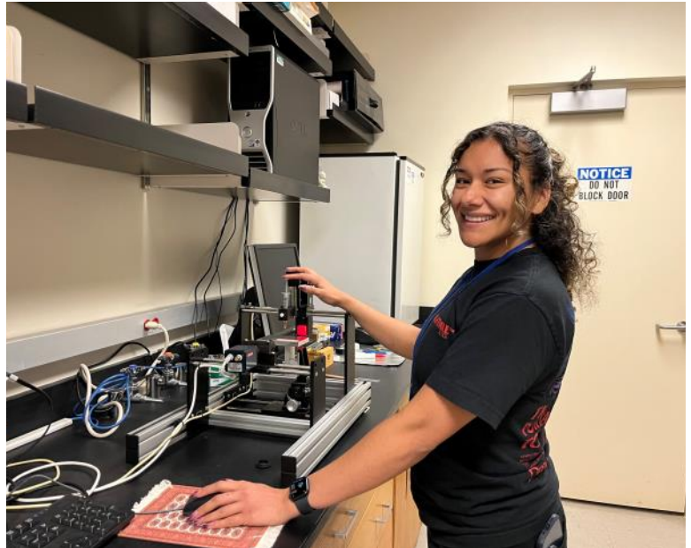
Veronica Gasca-Alcantar using a goniometer to measure the curve of a waterdrop (photo by Nicole Damon).
