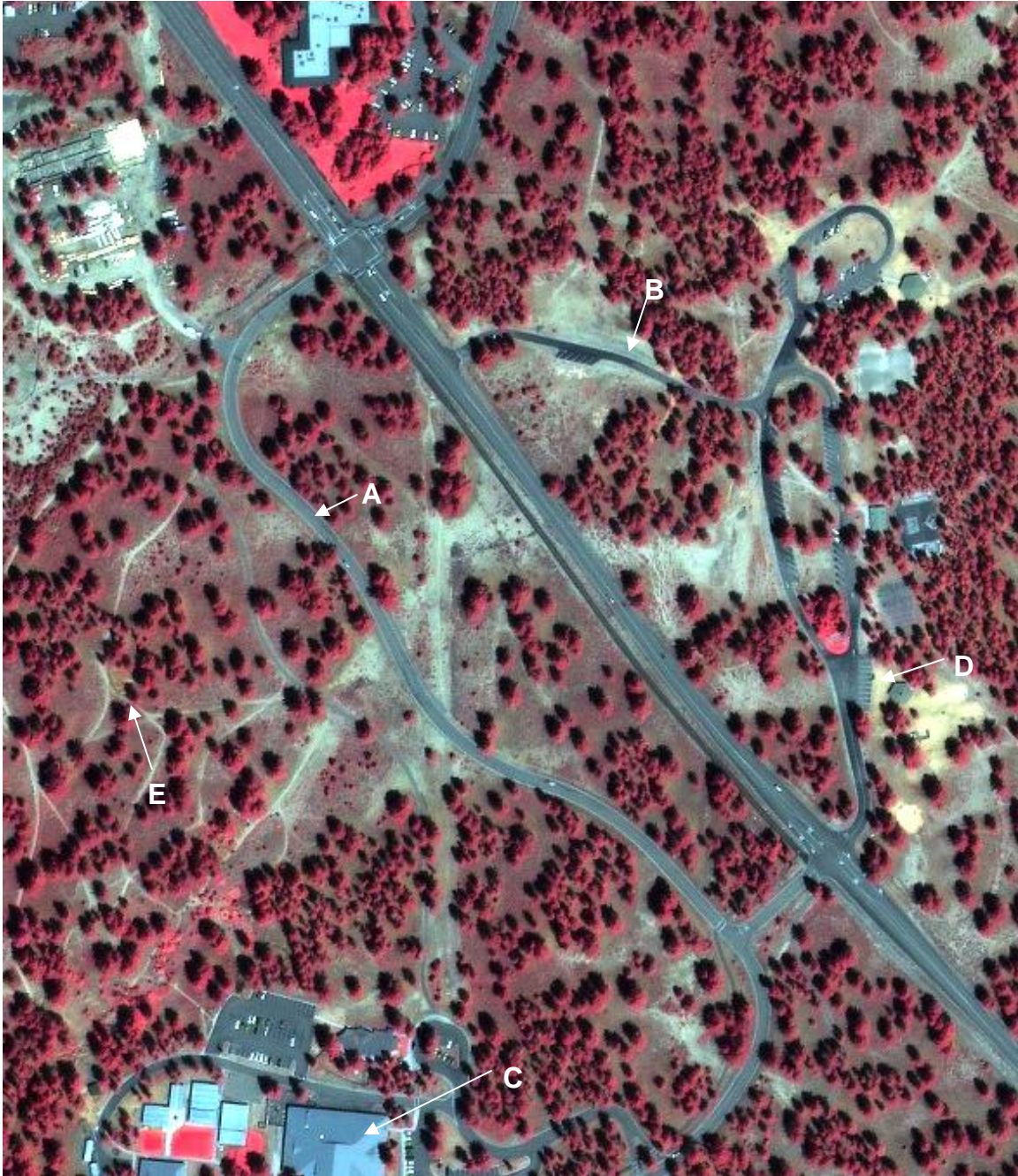
Figure 4. Examples of features at functional level III impervious cover. The illustration uses 2002 Space Imaging Ikonos imagery. A = hard/permanent/transportation; B = soft/permanent/transportation; C = hard/permanent/structure; D = soft/permanent/halo; E = soft/permanent/recreation.
