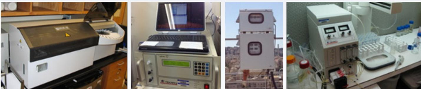
Pictures, from left to right: Nippon Mercury analyzer, Tekran 2537 and 1130/1135 analyzers; and water analyzer system.
