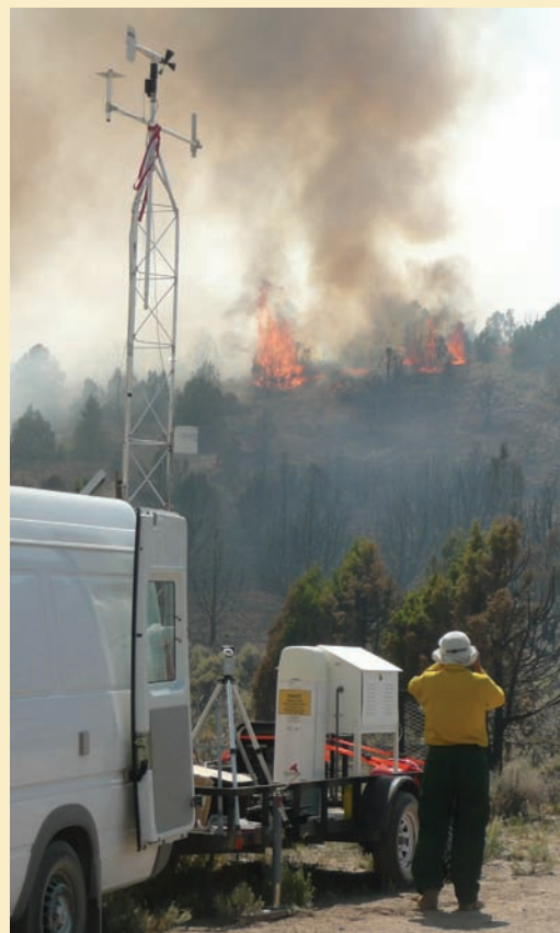
DRI's Portable Environmental Monitoring Station was deployed to measure emissions from the Upper Gleason Controlled Burn east of Ely, Nevada.
