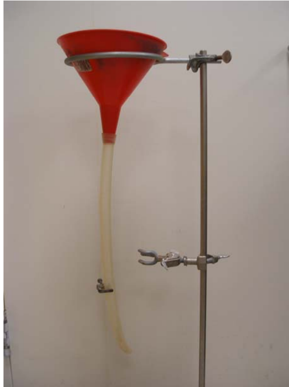
Figure 3.2: Funnel setup used to pack soil columns.
