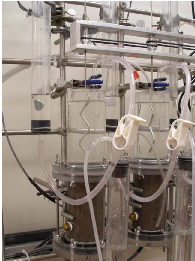
Figure 3.4: Stirring device used for soil column testing.
