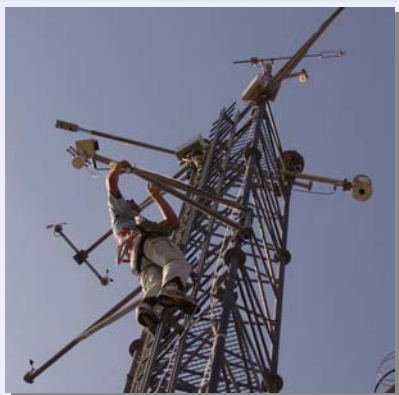
Daniel Obrist installing sampling filters and lines for measurement of ambient atmospheric mercury concentrations.
