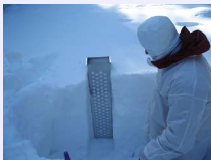
David Simeral taking snow samples looking for traces of the silver (seeding agent) in the Snow Range, WY.
