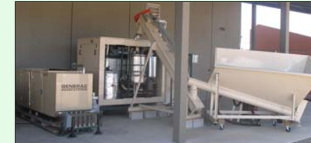
Figure 8: The Biomax 15 produces 15 kW of electrical power by burning syngas from gasification of biomass in a generator.
