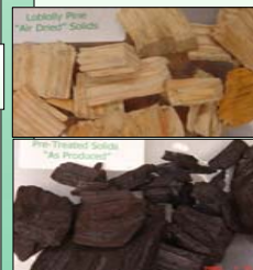
Figure 4: Loblolly pine chips before and after pre-treatment
