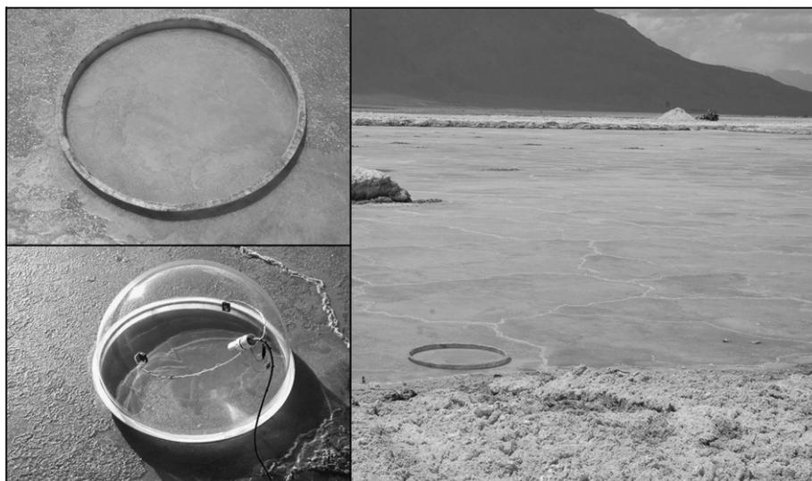
**Fig. 3.** Images from brine sampling at Site 2. Counter clockwise, starting from upper left is Site A with fiberglass ring emplaced into the floating brine crust that has healed completely after one hour, the chamber is shown atop the fiberglass ring during a measurement of Site B, and a fiberglass ring is in situ in Site A on the edge of a large salt encrusted pond.
